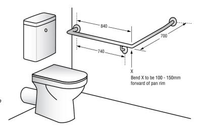
This product is AS1428.1 compliant (accessible compliant) when installed in accordance with the guidelines.
